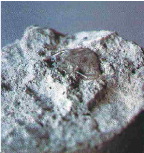
Water & contained salts or acids are unable to penetrate Non-Absorptive “Caltite” or “3CC” System concrete.
